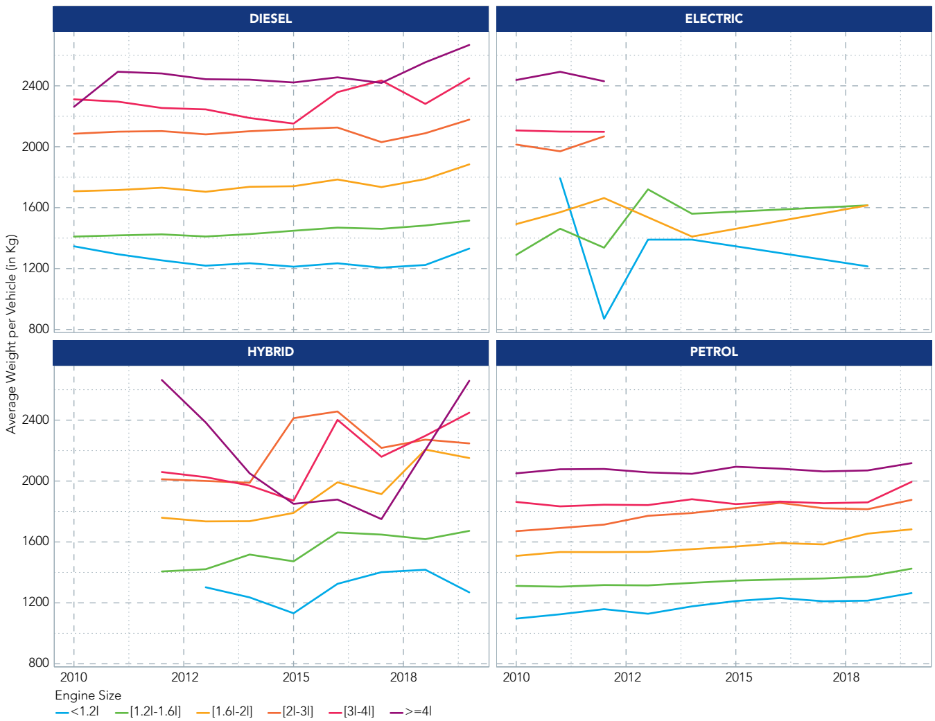
Figure 7: Average weight of vehicle vs fuel type and engine size in cm 3 across the EU fleet to 2018
