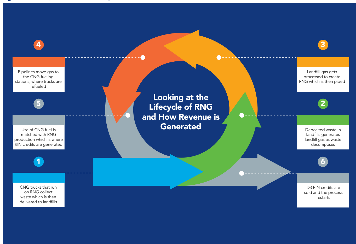
Figure 5: The lifecycle of RNG and how it generates revenue for waste companies
