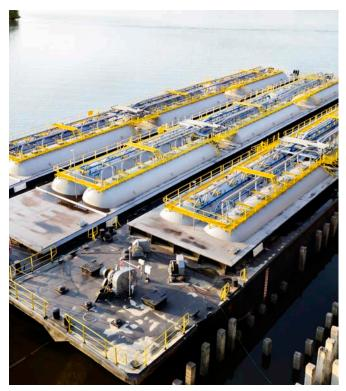
Tank barges primarily carry liquid, solid or gaseous commodities or cargoes in bulk along rivers and inland waterways.
